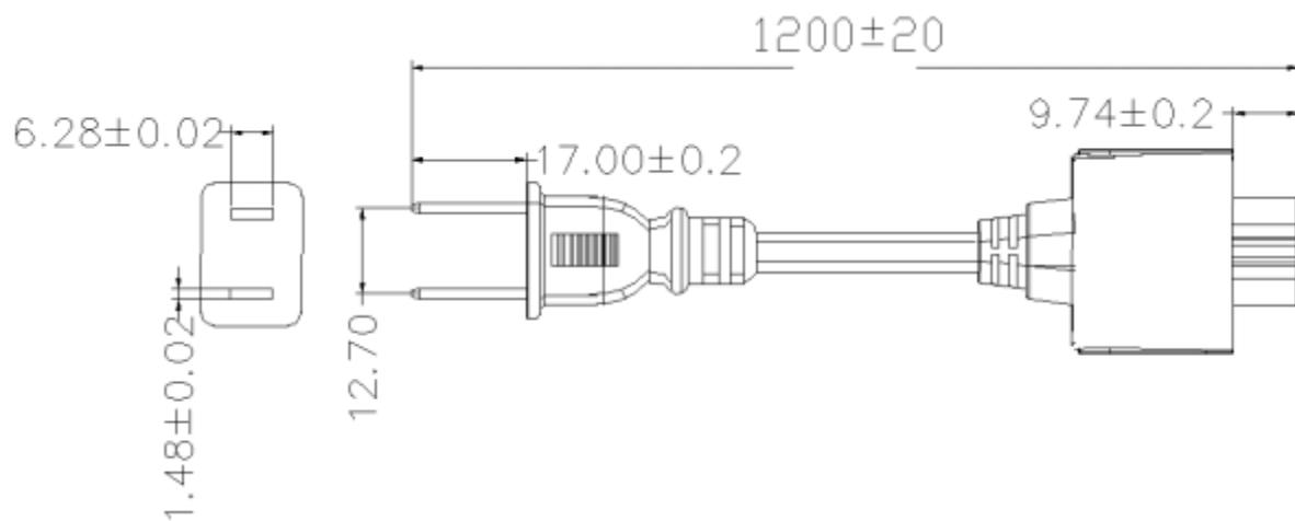
11.2. UK/SAA/EU/UL Change the plug (英规/澳规/欧规/美规, 可更换插头)
